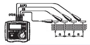
Useful for optimum earthing system design and location, to avoid extra cost of re-working electrode installation. Also for geological and archaeological investigations, etc.
