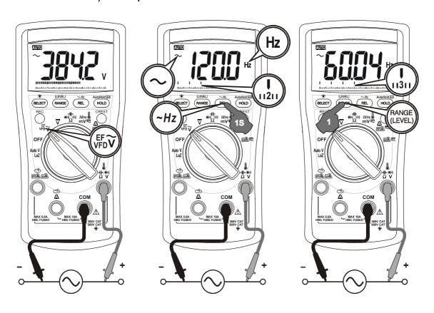
**NOTE:** It is recommended to start testing with the selected available function on the signal-under-test in auto-ranging mode before activating the ~Hz function for an appropriate trigger level automatically. If the ~Hz reading is unstable, manually select lower sensitivity to avoid possible electrical noises. If the reading shows zero, manually select higher sensitivity for the measurement.
