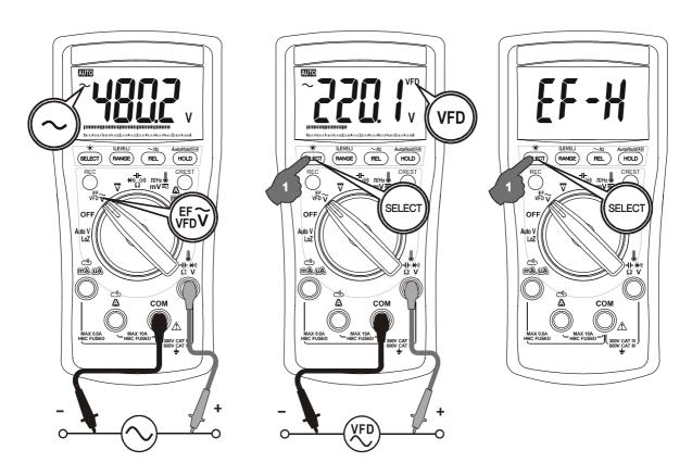
EF-Detection defaults to "EF-H", the High sensitivity, when it is ready. If it is too sensitive for your applications, short-press the (LEVEL) button to toggle to EF-L, the
